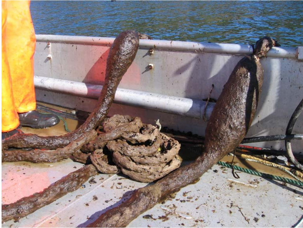
Figure 8: March 6 2008 – Intact polyester-cotton (50:50) sleeving (PC-ES) - note the tendency for the seed to move upwards to form balls at the top of the sleeve.
