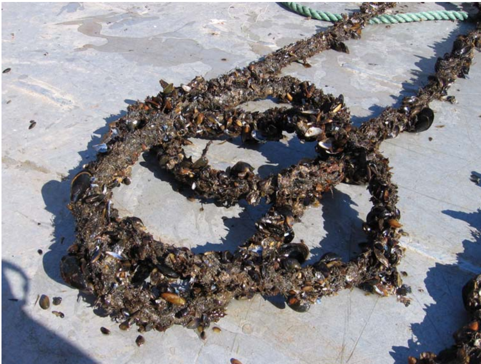
Figure 9: March 6 2008 - Polyester-cotton sleeving (28:72) (PC-RN) starting to break down – the mussels were creating holes in the mesh.
