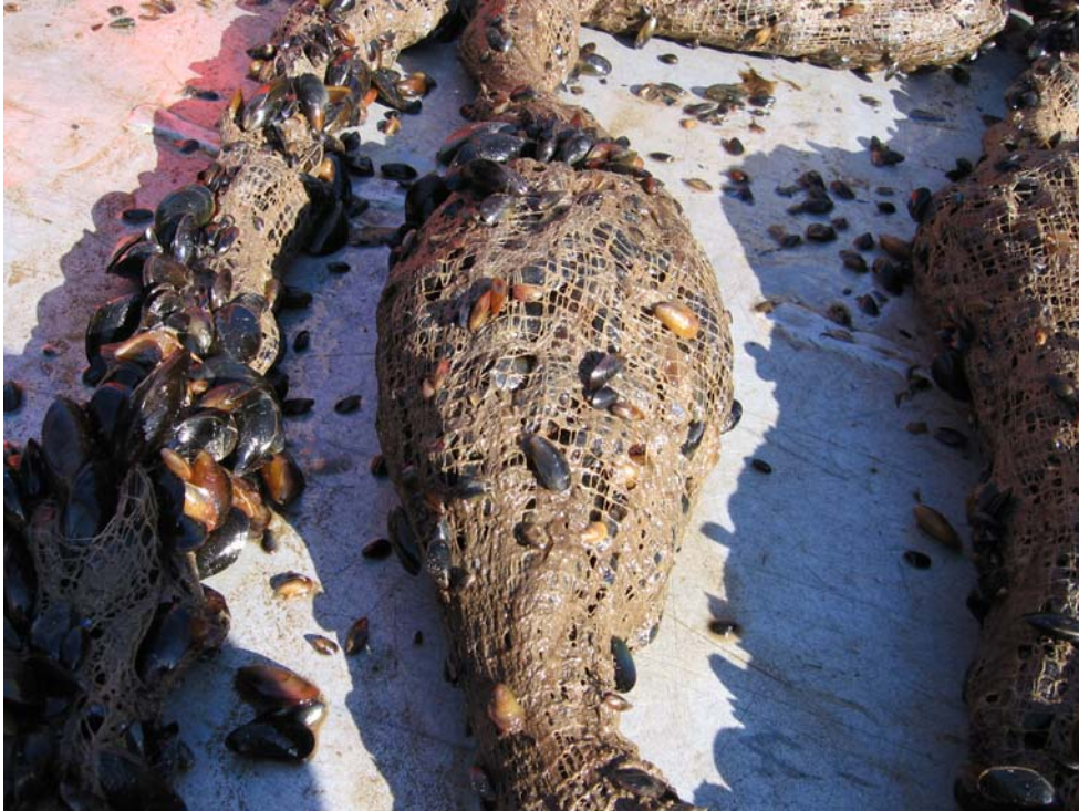
Figure 9: March 6 2008 - Polyester-cotton sleeving (28:72) (PC-RN) starting to break down – the mussels were creating holes in the mesh.
